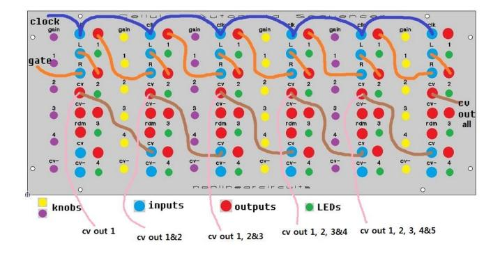
In the above patch, all of the neighbourhoods run off the same clock signal. Just one gate signal is used and patched through to activate every neighbourhood. The CVs are chained and summed outputs can be used elsewhere in the synth.
