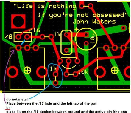
place 1k on the /16 socket between ground and the active pin (the one you solder the wire to) (easiest option!)
