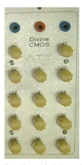
This panel layout only has the 2 inputs and a single output.
