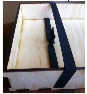
Best to drill holes (4mm dia), if not precut, for the handle with the lid on the case. Use the lasercut standoff as a guide. Find the centre of the case by measuring 220mm in from either side. Place the standoff over the centremark and use a pencil to mark out the holes. Drill the 4mm holes for the screws. The screws need to be cut/broken off, to
