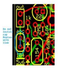
I did not have a 1k pot for the BD decay, so used a 10k. Much of the range is useless, so if using a 10k pot, place a resistor across the two solder points to reduce the total resistance, 1k5 to 2k2 would suit. If you have a 1k pot, do not do this mod, it is only if you cannot find a 1k pot and use a 10k. See pic.
