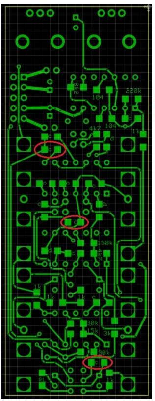
do not install leave empty 2. Replace 10k with 22k, this removes a dead zone at the bottom of the rate pot
