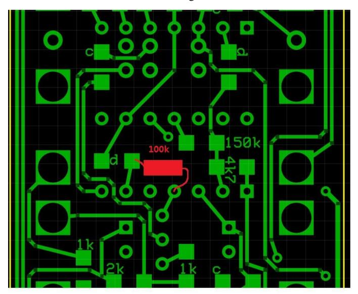
add 100k between the 10k (d) and pin4 of the TL074 (+V). You should be able to angle a 1206 resistor across the gap with the corners reaching the points it needs to be soldered to.
