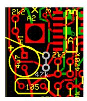
When the circuit is built, turn it on and measure the voltage of the signal at **pin 1** of the TL074 (A) next to the 47k resistor. Ideally use an oscilloscope and look at the lovely noise, possibly a multimeter will work as the noise is quite solid and may look like DC. You can expect get a voltage of 0.2 to 1.2V. Whatever you get, assuming you want noise levels of 5-6V, use this equation to determine the resistor:
