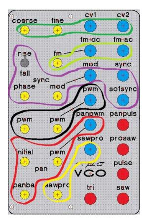
**GREEN** - The Coarse and Fine pots are fairly obvious. CV1 and CV2 are 1V/Oct inputs and are happy to accept any control voltage.
